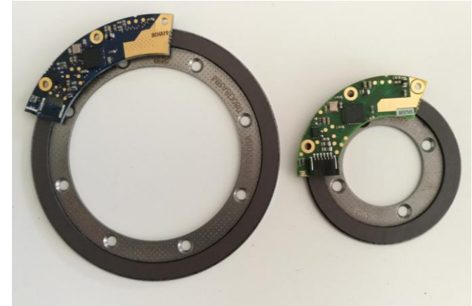
Magnetic off-axis absolute encoders in different sizes as used in ARMAR-6
