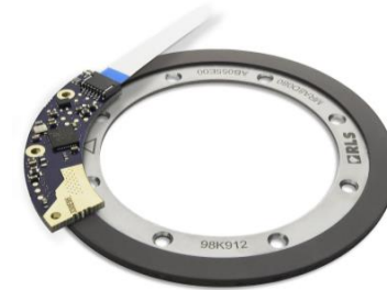
Magnetic off-axis position sensor
