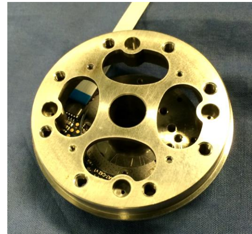
Encoder-based torque sensor
