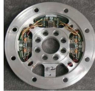
Spoke wheel type torque sensor of the DLR light-weight arm
