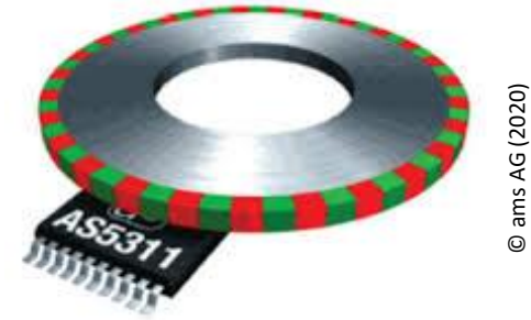
Magnetic encoder disk with quadrature encoder IC
