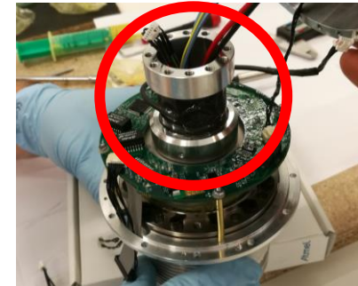
Torsional shaft type torque sensor in a sensor-actuator-controller unit of ARMAR-6
